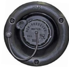
Fresh Water Gravity Fill Inlet
