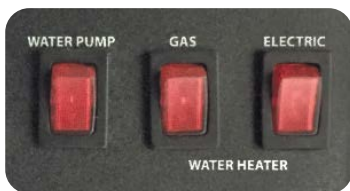
Water Pump & Water Heater On/Off Switches
