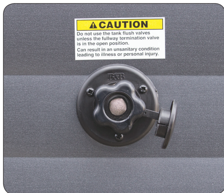
Black Tank Flusher Inlet is located on the off-door side of the RV.
