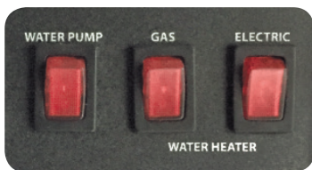
Water Pump & Water Heater On/Off Switches
