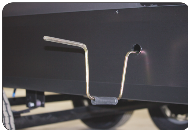
Slideout Override Access Hole & Crank Handle Extension
