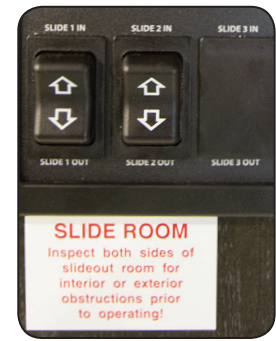
The Slide Room Switches are located inside the RV, on the Command Center.
