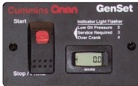
The Generator Remote Switch is found on the Command Center
