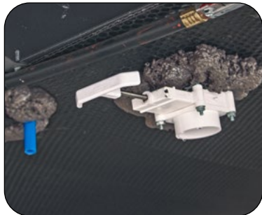
The Fresh Water Holding Tank Gate Valve is located under the RV
