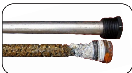
Brand New Anode Rod (top) Corroded Anode Rod (bottom)
