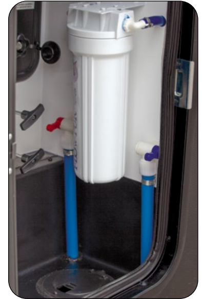
Water Filter and Low-Point Drains are located in the Universal Docking Station
