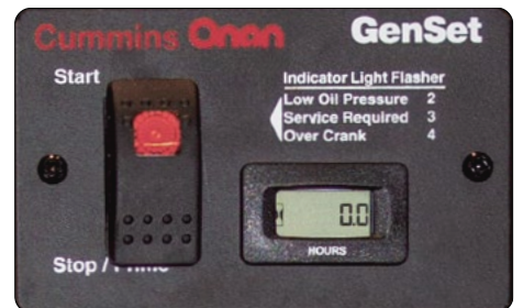
On the S-Class, the Generator Remote Switch is found on the Command Center
