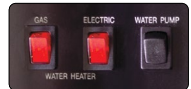
Water Pump & Water Heater On/Off Switches
