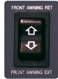
The Patio Awning Switch is located inside the RV, on the Command Center
