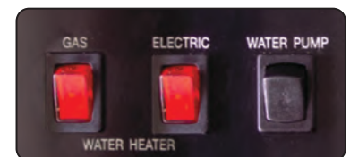
Water Pump & Water Heater On/Off Switches
