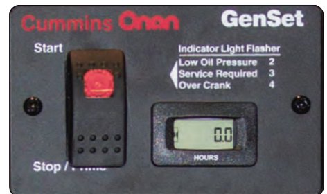
On the S-Class, the Generator Remote Switch is found on the Command Center
