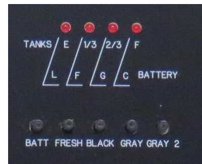
Photo shows a typical monitor panel section, located on the command center inside the RV.
