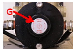
Typical protective seal, located on the end of the motor attached to the hydraulic reservoir.
