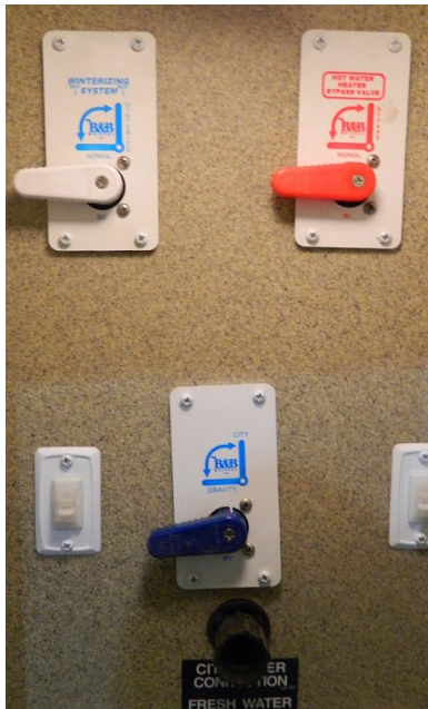
Typical valve positions for gravity water fill usage (connect hose to black inlet)
