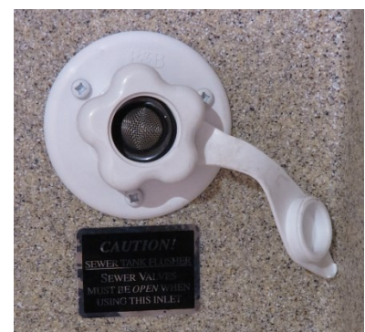
Sewer tank flusher, located in the utility center on the right-hand side.
