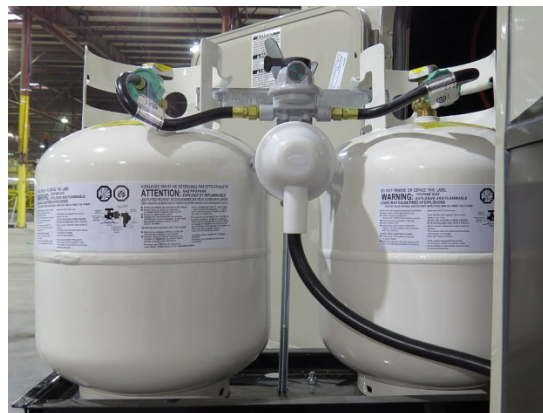
This photo shows a typical configuration of the two main working 20 lb. cylinders located in the front off-door side compartment. (The front door side compartment contains a single spare cylinder that is not connected to the RV propane system; it is for storage purposes until needed only.)
