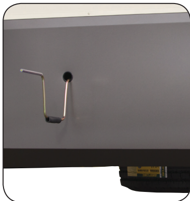
Spare Tire, Access Hole & Crank Handle Extension
