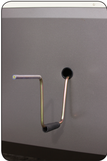
Slideout Override Access Hole & Crank Handle Extension
