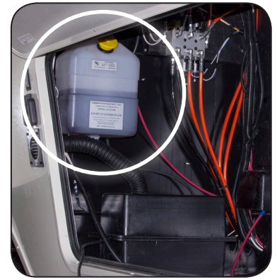
The Hydraulic Fluid Reservoir is located in the Front Compartment. It supplies fluid to both the Hydraulic Landing Gear & the Hydraulic Slide Systems.
