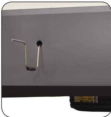
Spare Tire Access Hole & Crank Handle Extension
