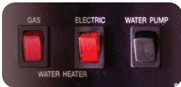
Water Pump & Water Heater On/Off Switches
