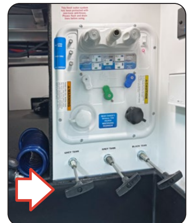
The Black Tank & Grey Tank Drain Valve (or dump valve) handles are located below the Nautilus P4 Water Panel.
