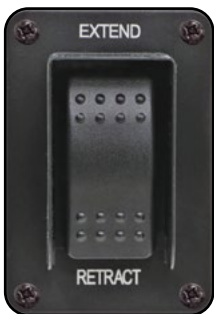
Power Stabilizer Jack Manual Control Switches Are Located on the RV's Off-Door Side.
