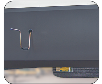
Spare Tire, Access Hole & Crank Handle Extension
