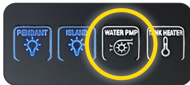
Water Pump On/Off Switch
