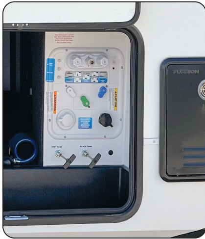
The Nautilus P4 Water Control System Is Located Inside The Off-Door Side, Forward Compartment.
