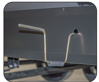
Slideout Override Access Hole & Crank Handle Extension
