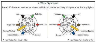
Typical 7-way wire harness wiring diagram
