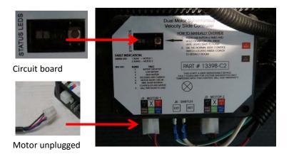
Typical Schwintek InWall slide system slide controller, generally located in the front pass-through storage area (bedroom slide) or near the living area slide(s) inside a cabinet.
