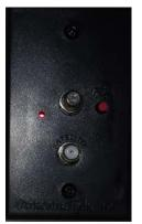
Typical TV signal booster, the ON/OFF red button is located on the right side of the face plate.
