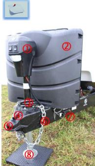
Typical A-frame locations: 1 – Power tongue jack 2 – LP bottle cover 3 – 7-way Wire Harness/Connector Plug 4 – Tongue jack coupler latch 5 – Tongue jack coupler
