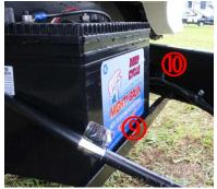
Typical A-frame locations, cont: 9 – Battery box location 10 – In-line fuse
