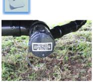
*Typical sewer outlet connection, located on the off-door side.*
