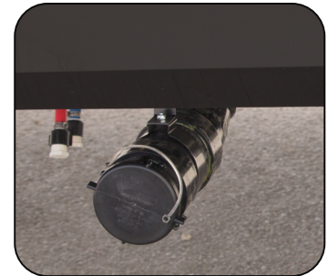
Sewer Outlet Connection Is Located Under the RV on the Off-Door Side
