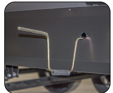
Slideout Override Access Hole & Crank Handle Extension
