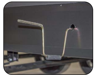
Slideout Override Access Hole & Crank Handle Extension
