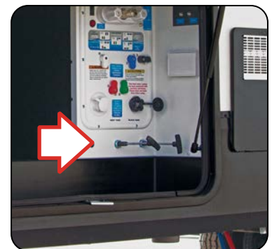
The Black Tank and Grey Tank Drain Valves (or dump valves) are located below the Nautilus P1 Water Panel.
