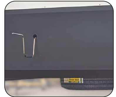
Spare Tire, Access Hole & Crank Handle Extension
