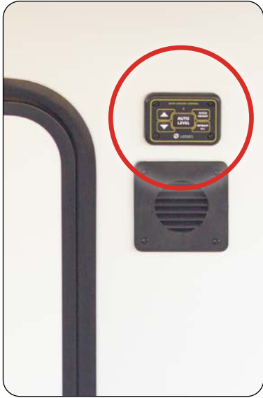
The Auto Leveling Control Touch Pad is located on the Front of your FW
