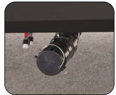
Sewer Outlet Connection Is Located Under the RV on the Off-Door Side
