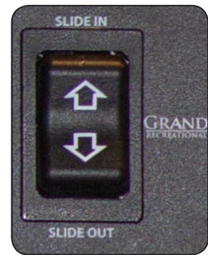
The Slide Room Switch Is Located Inside the RV, on the Command Center.
