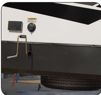
Spare Tire Access Hole & Crank Handle Extension
