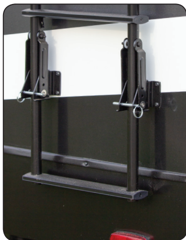
Roof Ladder Locking Pins
