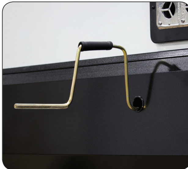
Slideout Override Access Hole & Crank Handle Extension
