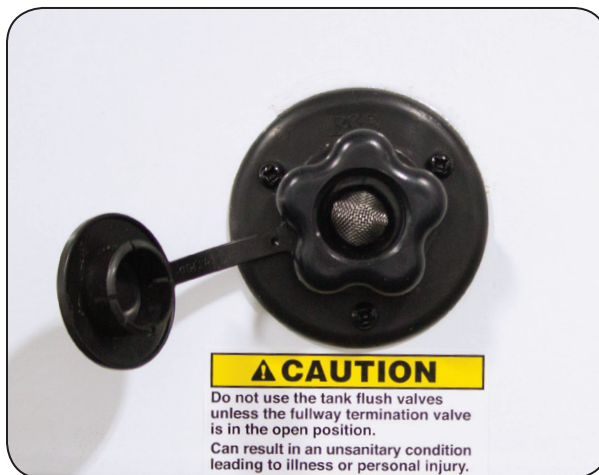
Black Tank Flusher Inlet Is Located on the Door-Side of the RV.
