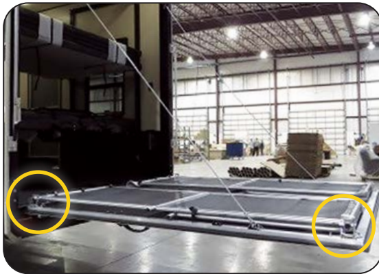
Patio Rail Front & Rear Brackets with Locking Safety Pins
