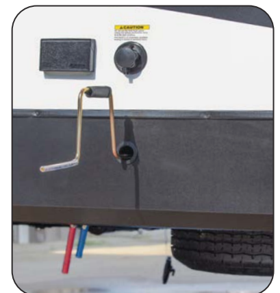
Spare Tire Access Hole & Crank Handle Extension
