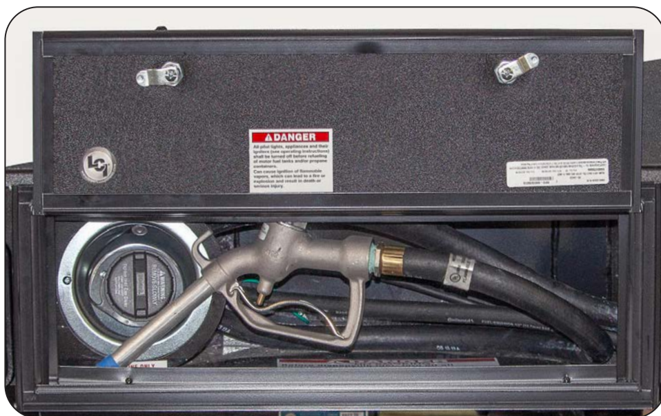
The Fuel Station is Located on the Exterior Off-Door Side
