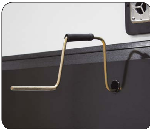
Slideout Override Access Hole & Crank Handle Extension
