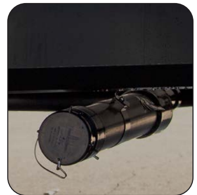
Sewer Outlet Connection Is Located Under the RV on the Off-Door Side
