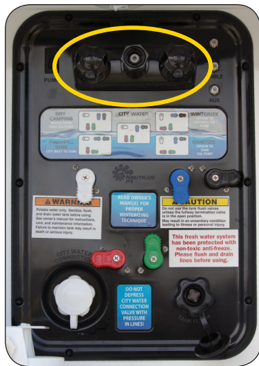
Exterior Spray Port
