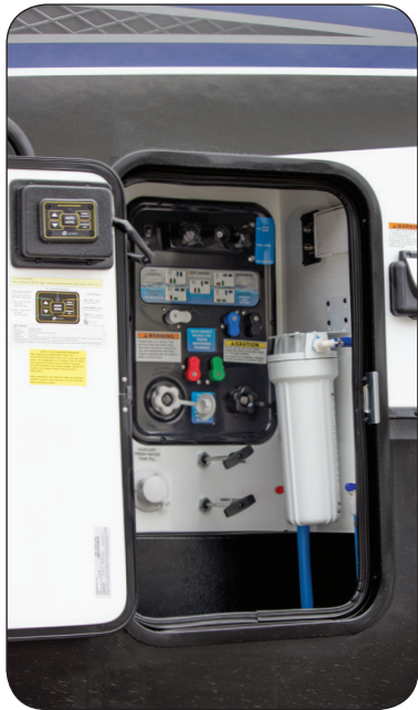
The Nautilus P1 System Is Located On The Forward Off-Door Side
