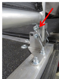
6. Insert the safety pin (removed in step 4) to the topmost position as shown to secure the side patio gates vertically.
