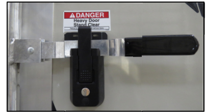
Photo shows typical ramp door handle and lockset
