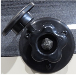
Typical sewer tank flusher, located in this instance on the exterior RV sidewall.
