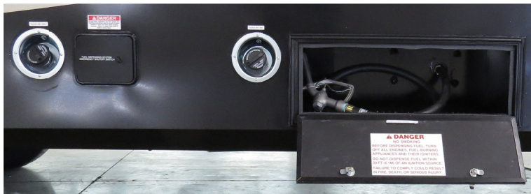
Typical fuel system, located on the exterior sidewall.
