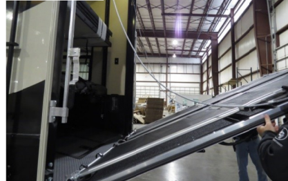
2a. Carefully lower and open the ramp door making sure both ramp door cable ends are fastened securely...
