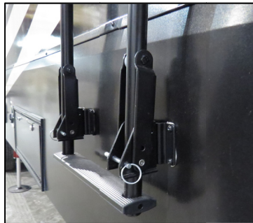
Photo shows typical roof ladder with locking pins in the closed (travel) position.
