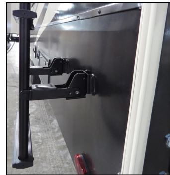
Photo shows typical roof ladder extended for normal use when the RV is parked
