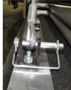
2b. ...by the safety pin at the ramp door bracket as shown above.
