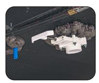
Fresh Water Holding Tank Gate Valve, located under the RV
