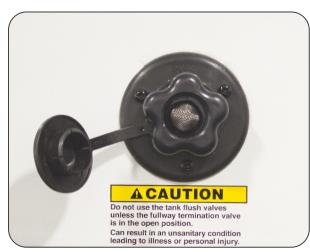
The Black Tank Flusher Inlet is located on the off-door side of the RV.
