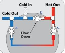
Valve Positions -Draining the Water Heater
