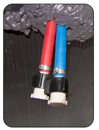
Low-Point Drain Valves located under the RV
