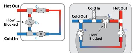
• During *Winterization* or *Sanitization*, turn the water heater bypass valves to the *Bypass* position shown below:
