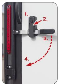
The *Rear Ramp Door* is easily operated by one person to give full access to the garage.
