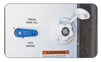
b. For normal city water use at a campground, turn the city water control handle as shown below:
